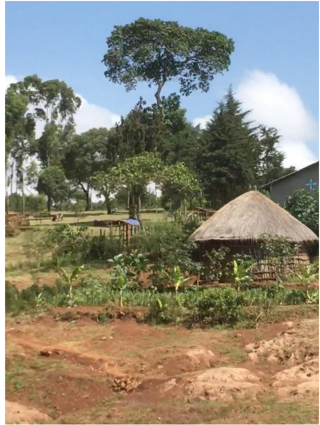
A homestead west of Lake Hawassa in Southern Province People. Right behind the round hut is a "modern house" with about 7x4 m. These houses are built of poles and encased with straminous clay.
